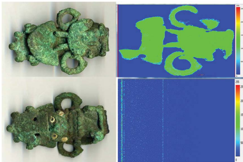
Figure 1. Left – Front and back views of the Moche Cast Figure. Right - Spatial X-Y view (top) and X-Energy view (bottom) of Moche imaged by SEM-EDS. The 3D volume contains 2048 spectral frames with spatial dimensions of 11,520 x 9,984 pixels per frame.
